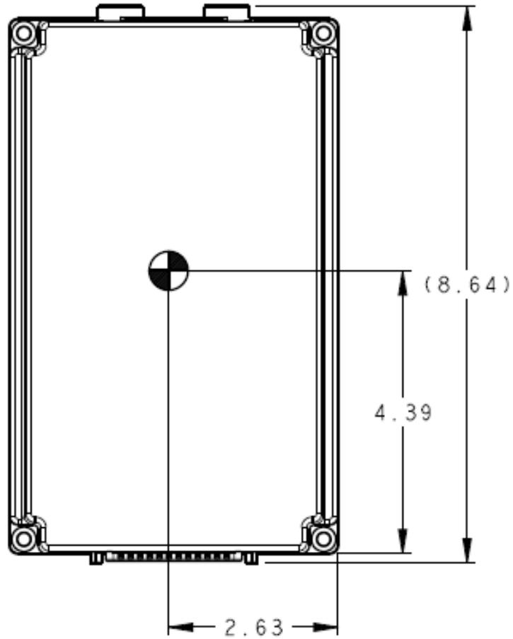
**Figure A-6 KG 71EXP Dimensions and Center of Gravity**
