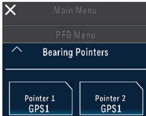
**Figure 7-8 Bearing Pointers Sub-Menu**
