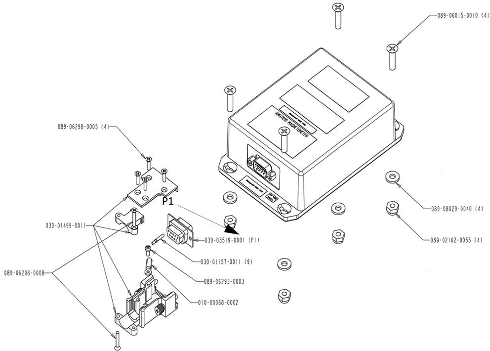
Figure 4-19 KDC 100EXP Data Connector Installation Diagram
