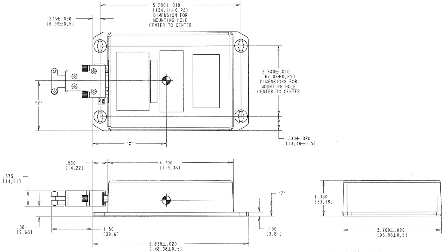
Figure A-11 KDC 100EXP Outline and Mounting Drawing (Sheet 1 of 2)
