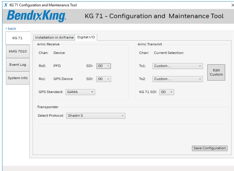
**Figure 6-50 CMT Page for Digital I/O Configuration**
