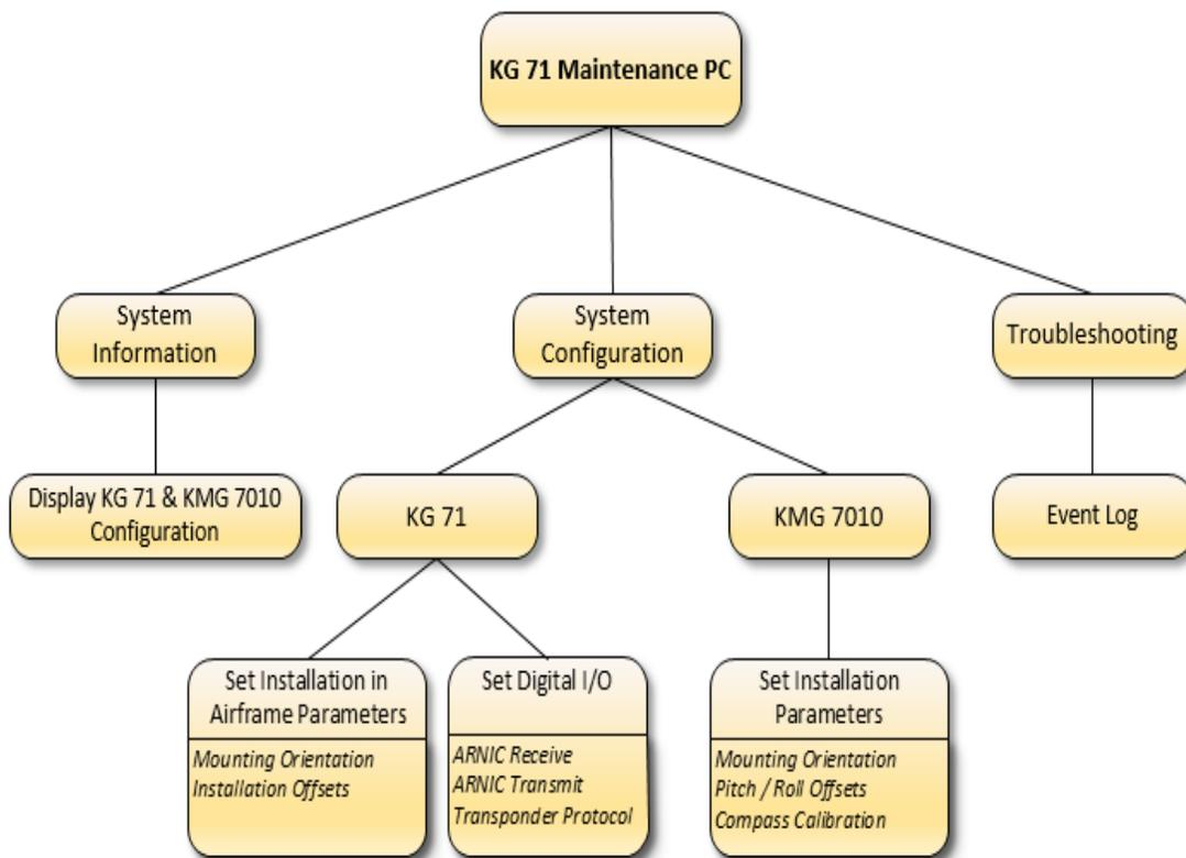
Figure 6-2 KG 71EXP Installation/Maintenance Functional Diagram
