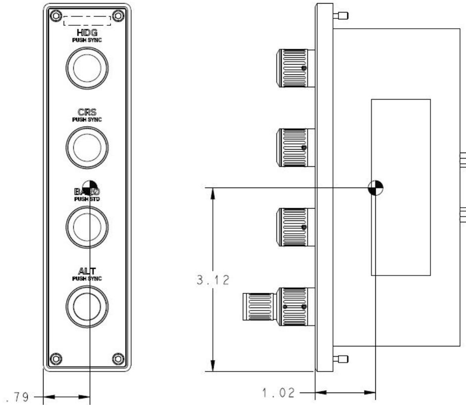
**Figure A-3 KCP 100EXP Dimensions and Center of Gravity - Portrait Orientation**
