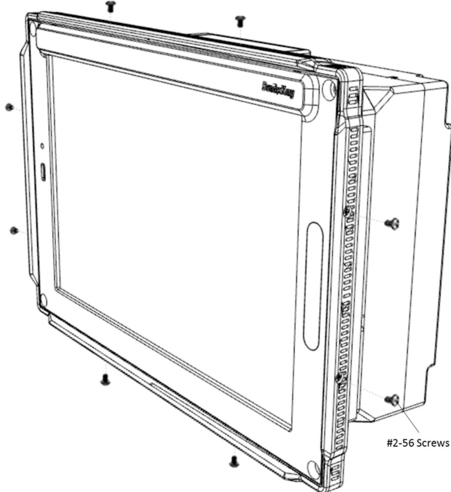
**Figure 4-10 KSD 100EXP Grip Installation (Sheet 2 of 2)**
