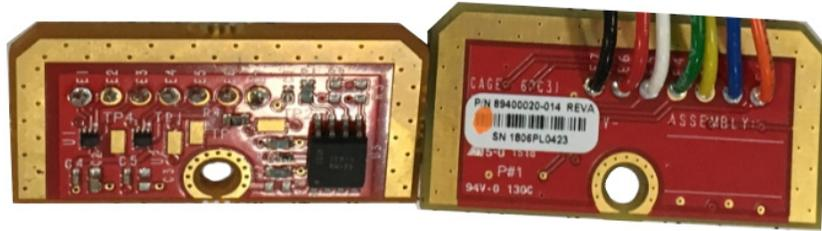
**Figure 4-7 Wired Configuration Module Circuit Card Assembly**
