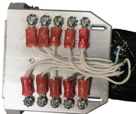
**Figure 4-8 Bottom Side of J2 Backshell**
