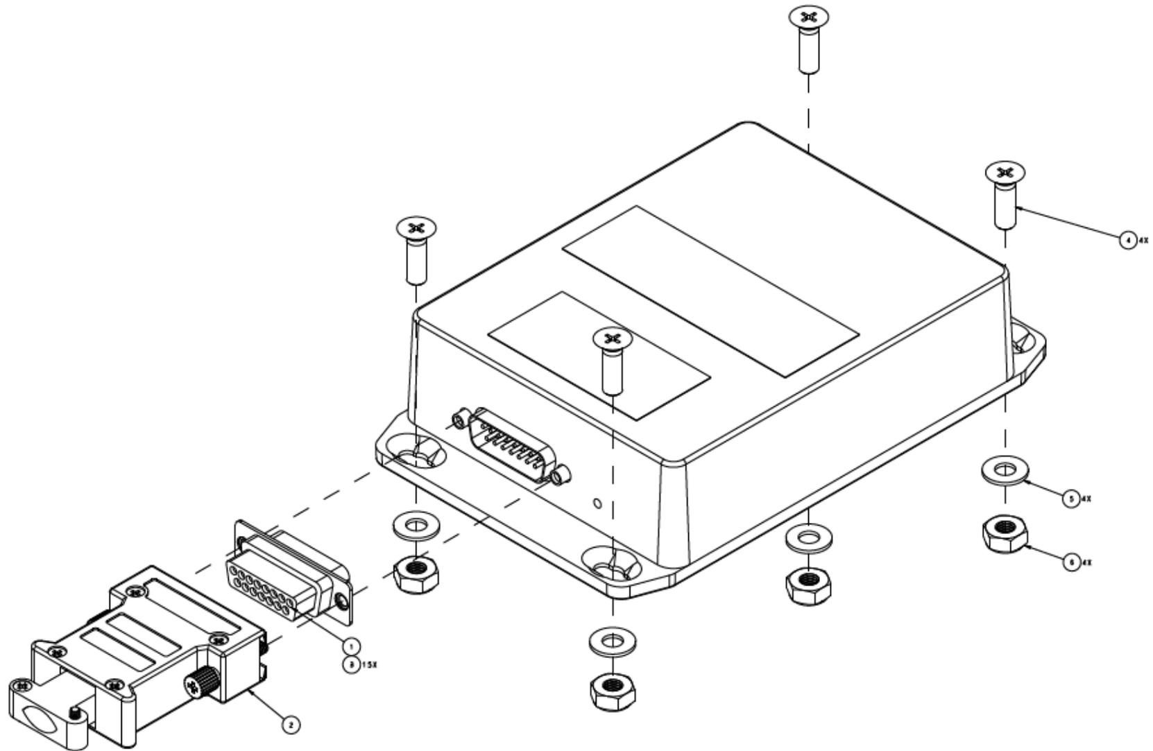
Figure A-12 KDC 100EXP Outline and Mounting Drawing (Sheet 2 of 2)
