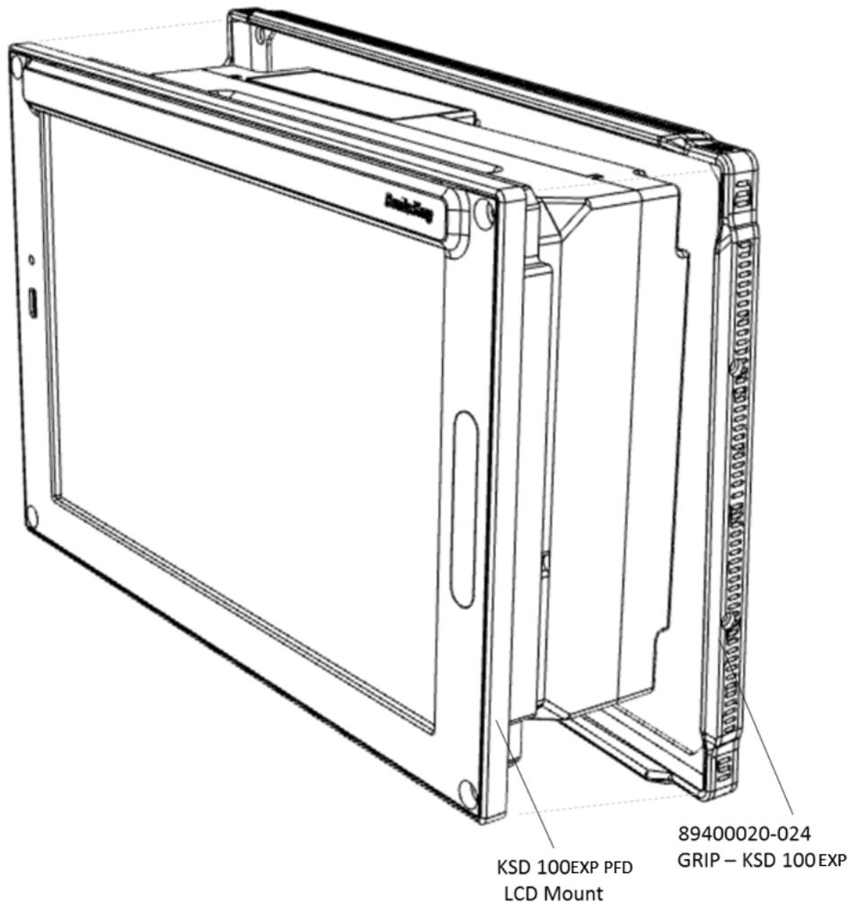
Figure 4-9 KSD 100EXP Grip Installation (Sheet 1 of 2)
