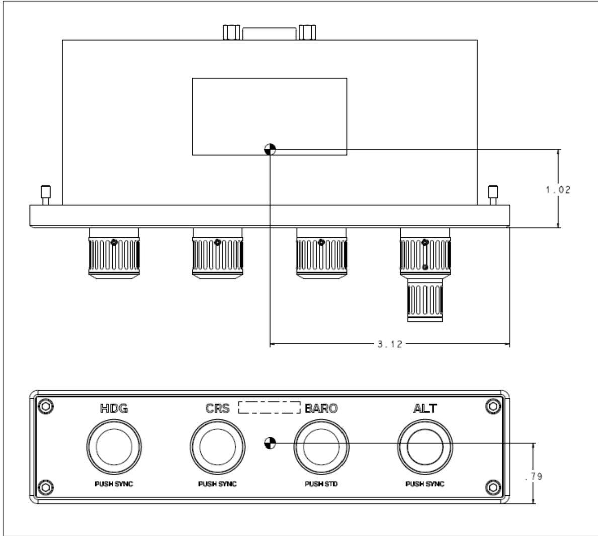
**Figure A-4 KCP 100EXP Dimensions and Center of Gravity - Landscape Orientation**
