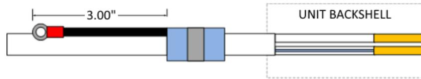
WHEN TERMINATING SHIELD GROUNDS TO THE OUTSIDE OF xVue Touch SYSTEM BACKSHELLS, IT IS RECOMMENDED TO APPLY THE SOLDER SLEEVE AS SHOWN IN THIS FIGURE. THIS IS TO PREVENT OVERCROWDING INSIDE THE BACKSHELL WHILE STILL PROVIDING AN ACCEPTABLE METHOD OF GROUNDING THE SHIELD.
