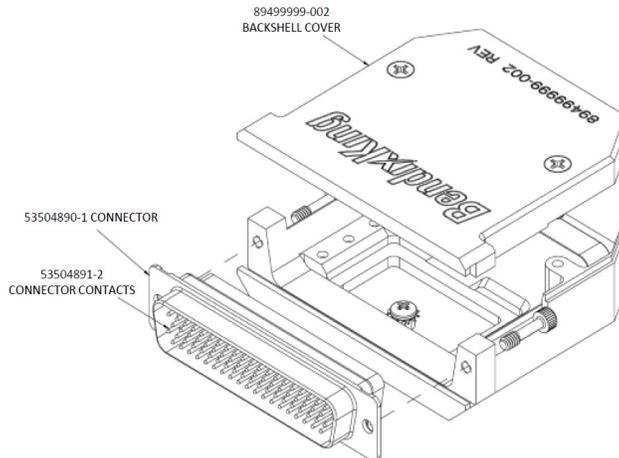
**Figure 4-3 KSD 100EXP J1 Connector Assembly**
