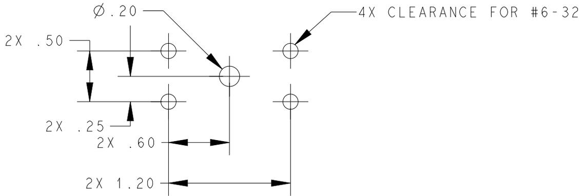
**Figure A-14 KTP 73 Mounting Hole Pattern**
