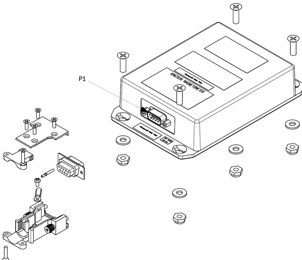
Figure 4-17 KMG 7010 Magnetometer Installation Diagram
