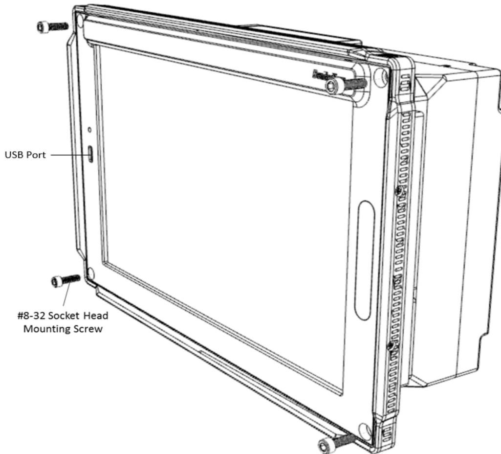
Figure 4-11 KSD 100EXP Installation
