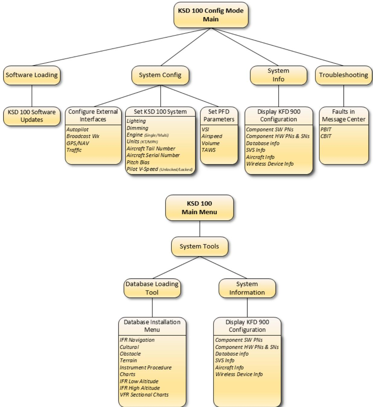
Figure 6-1 KSD 100EXP Installation/Maintenance Functional Diagram
