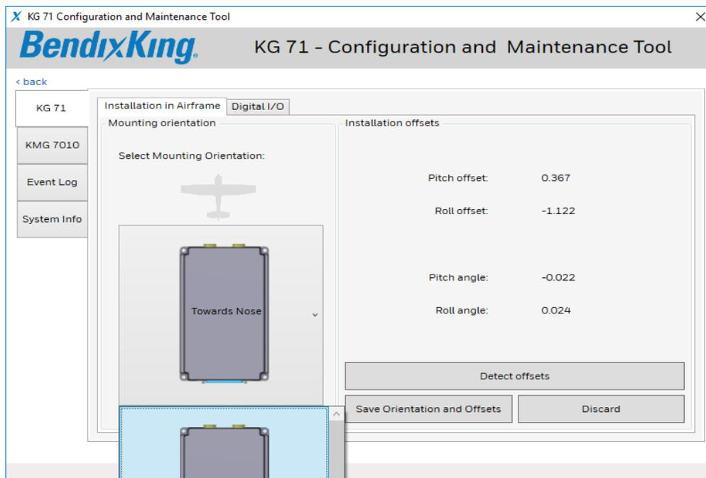
**Figure 6-48 KG 71EXP Orientation Drop-Down List**
