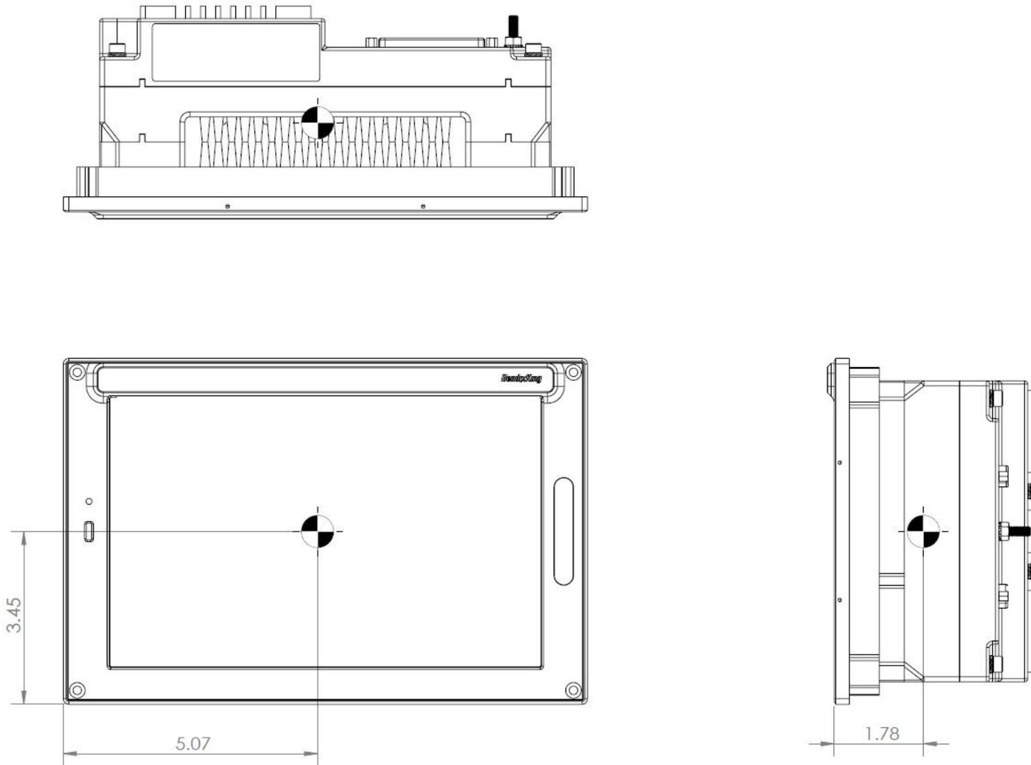
Figure A-1 KSD 100EXP Center of Gravity
