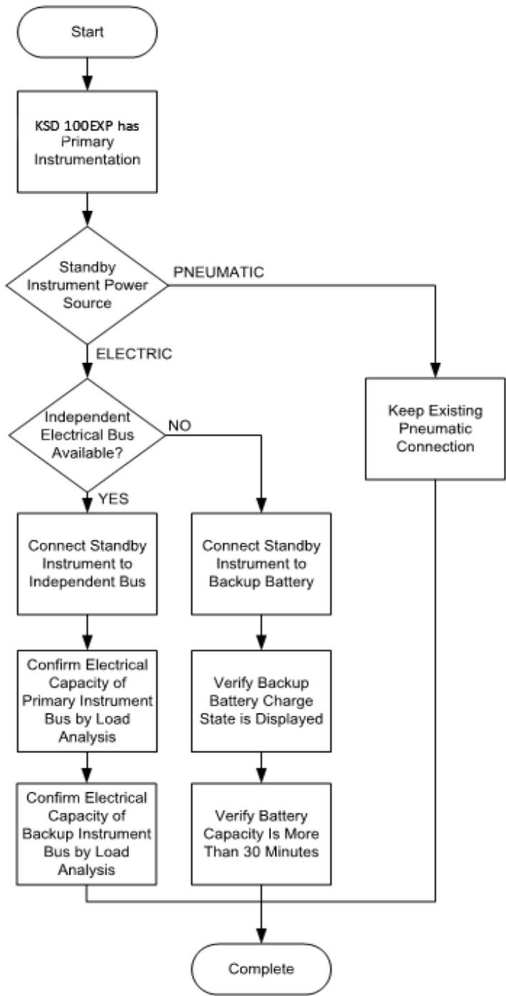
**Figure 2-3 Standby Instrument Power Requirements**
