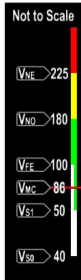
Figure 6-26 V-Speed Tape Illustration
