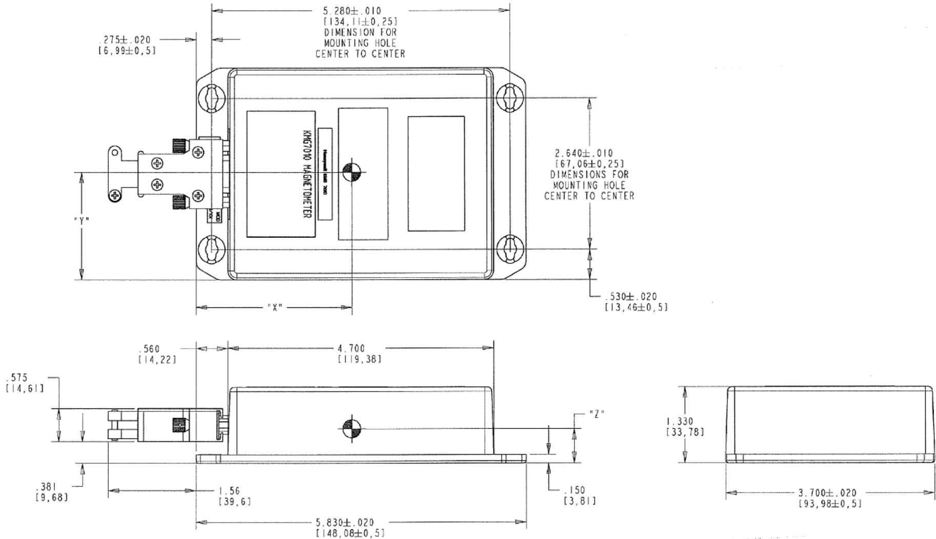
Figure A-8 KMG 7010 Outline and Mounting Drawing (Sheet 1 of 2)
