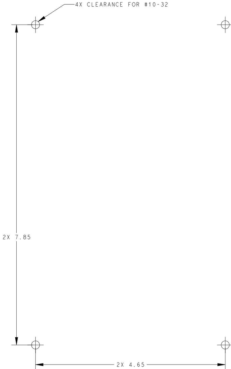
**Figure A-7 KG 71EXP Mounting Hole Pattern Diagram**
