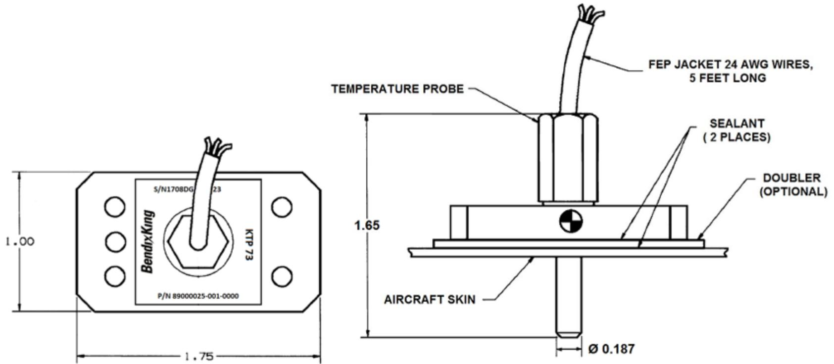
Figure A-13 KTP 73 Dimensions and Center of Gravity
