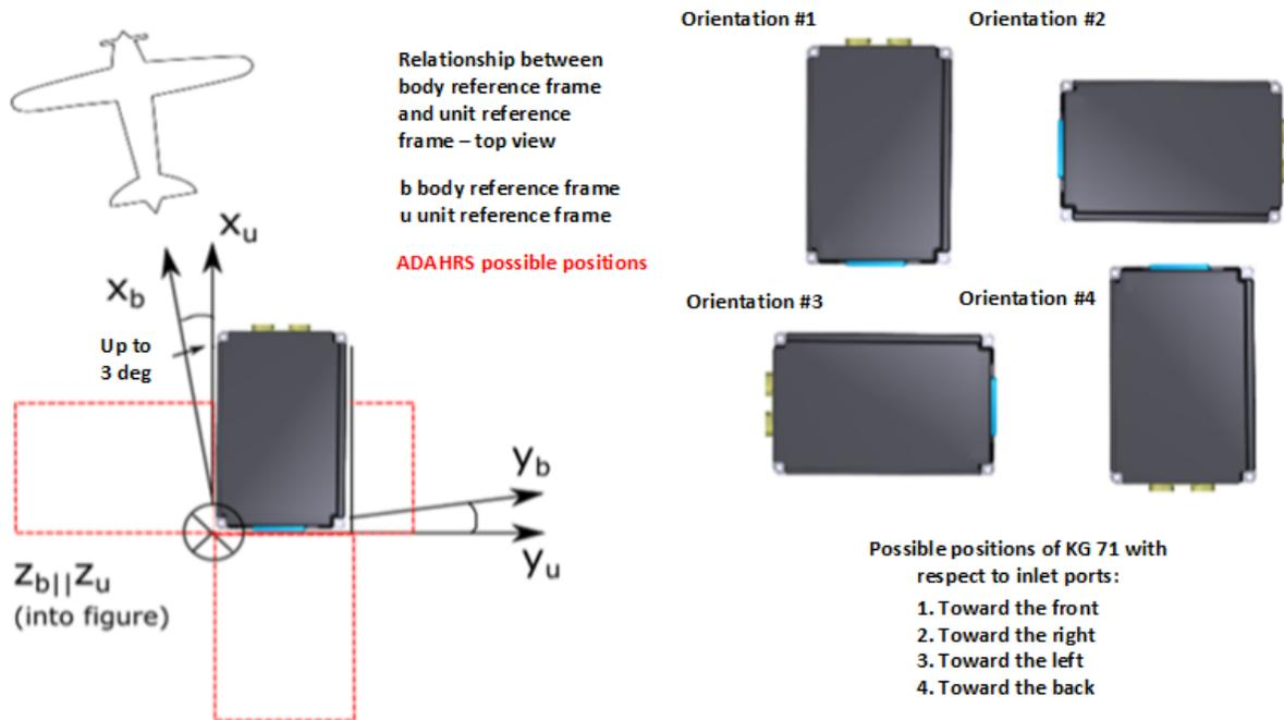
Figure 3-5 Supported KG 71EXP Installation Orientations
