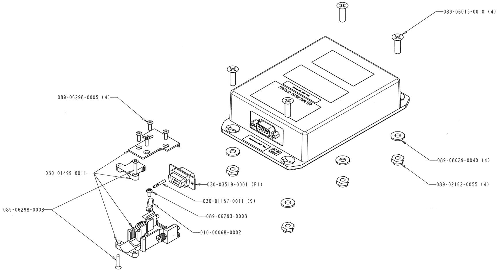
**Figure A-9 KMG 7010 Outline and Mounting Drawing (Sheet 2 of 2)**
