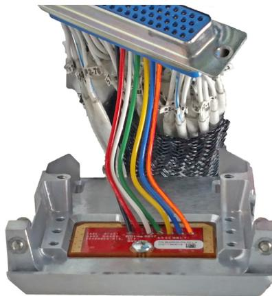
Figure 4-6 Configuration Module Inside J2 Backshell
