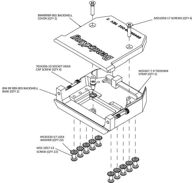
**Figure 4-2 BendixKing Backshell Assembly**
